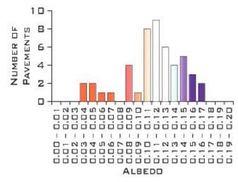
Over time, the average albedo of asphalt concrete is about 0.12
