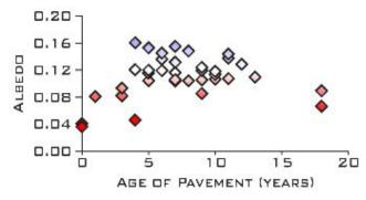
Over time, the albedo of asphalt concrete approaches 0.12
