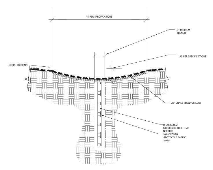
NOTES: DRAINCORE2 STRUCTURE CAN BE MULTIPLE LAYERS AS NEEDED
